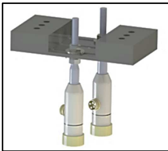
Measurement system for detection of RCF cracks (based on two differential eddy current probes)
