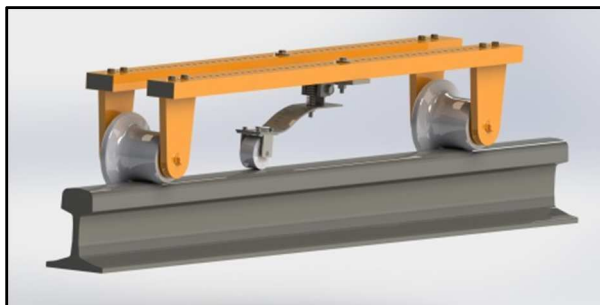
Measurement system for the device position (based on a multi-magnet wheel and a hall effect sensor)
